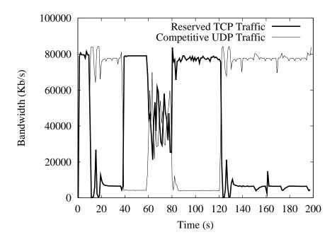
Figure 11. Performance achieved for a TCP flow in the presence of competing UDP traffic and host load, for various combinations of network and CPU reservation. We demonstrate GARA's ability to co-reserve multiple resource types.
