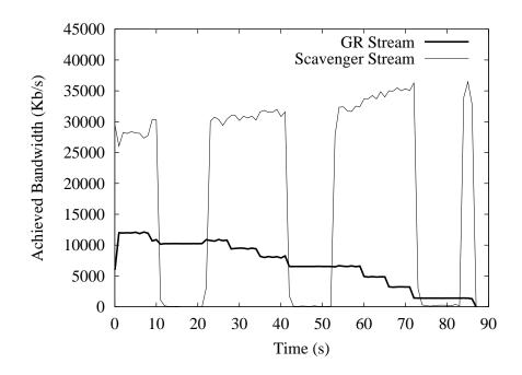
Figure 7. Performance achieved with a combination of a Guaranteed Rate service and a Scavenger service. While the Scavenger service reacts to periods of congestion, the Guaranteed Rate service remains stable. We see three periods of congestion: from 12-22, from 42-52, and from 72-82 seconds.
