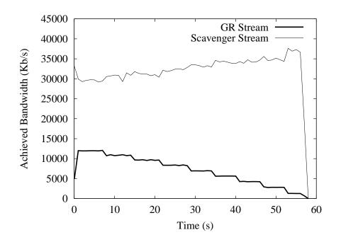
Figure 6. Performance achieved with a combination of a Guaranteed Rate service and a Scavenger service. We demonstrate that a bulk-transfer application with deadline is able to use a Guaranteed Rate service and in addition exploits unused Premium and Best-Effort capacity by a Scavenger service. See text for details.
