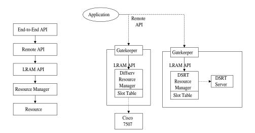
Figure 1. On the left, the principal APIs used within GARA. On the right, the principal components of the GARA prototype as instantiated for DS and DSRT (CPU scheduler) services, with our own resource manager and slot manager being used in both cases. In the DS case, commands are issued to a router while in the DSRT case commands are issued to a DSRT server (for tracking reservations).
