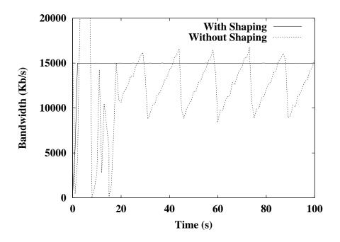
Figure 10. Achieved throughput for a Premium TCP flow exceeding the reservation. This time, the SACK-option was enabled. The average achieved throughput was 11992 Kb/s without shaping and 14448 Kb/s when shaping was activated. See text for details.
