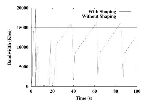
Figure 9. Achieved throughput for a Premium TCP flow exceeding the reservation. The SACK-option was disabled. The average achieved throughput was 9440 Kb/s without shaping and 14320 Kb/s when shaping was activated. See text for details.
