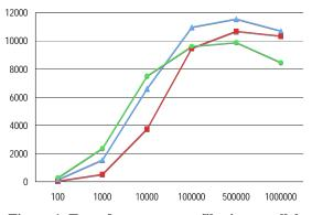
Figure 1. Transfer rate versus file size parallel TCP/IP LAN
